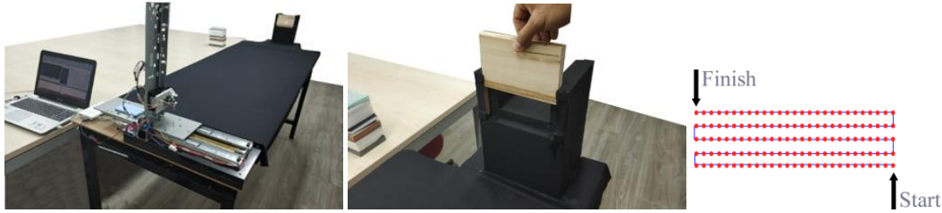
Figure 6. Experimental setup and the motion pattern of the Cartesian robot used for measuring
