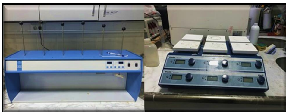
Figure 1 Laboratory scale Jar Test setup
