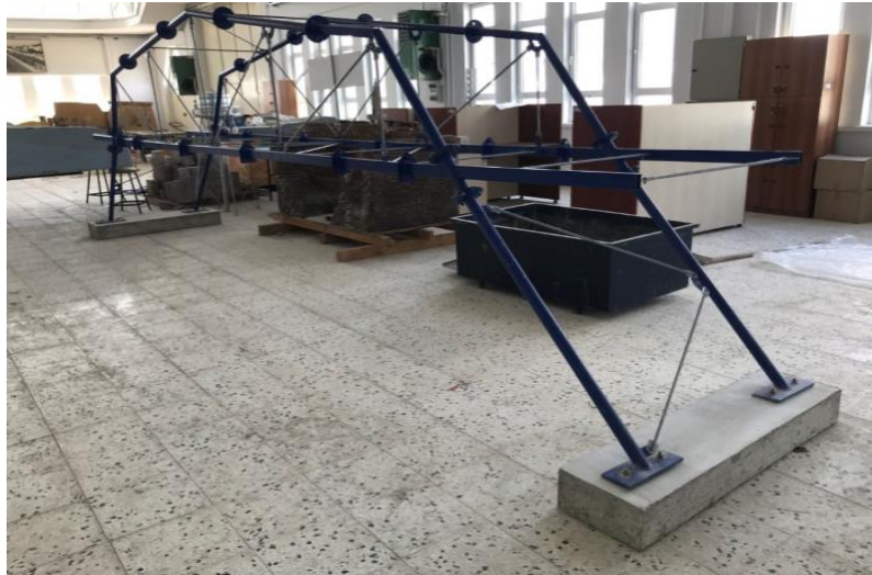
Fig. 1. Model steel bridge with diagonal bars in laboratory
