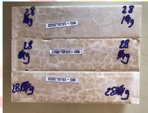
Figure 4. The cracks observed in M_1 samples at 28 days.
